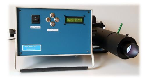
in a continuous "On" mode. Here the lamp is on in continuous mode with yellow background in the display.
