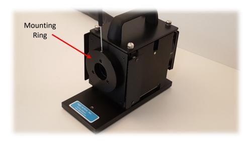
3. Slide the shroud on to the mounting ring.
