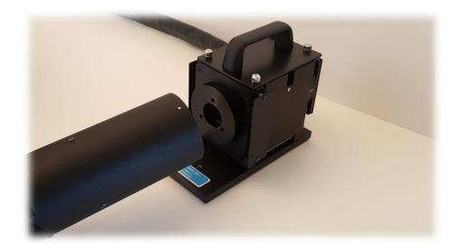
4. Install the top screw first. Tighten ¼ turn when the screw head contacts the shroud surface.
