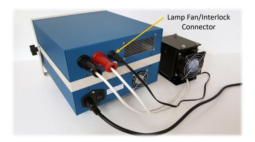
14. Connect the female end of the AC power cord to the back of the Power Supply and plug the male end into a 3-wire **grounded** wall receptacle. **DO NOT** use an ungrounded outlet at any time. Turn the "Power OFF/ON" switch to the ON position. The fans for the power supply and lamp holder will turn on and the LCD Display will illuminate. If any of the fans are not working, turn OFF the power supply and resolve the problem before continuing.
